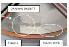
When the bearing was removed from the machine, all the thrust pads showed some signs of distress, as shown in Figure 1.
