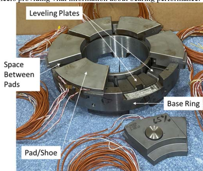
Figure 1: Flooded 65% offset steel bearing.
